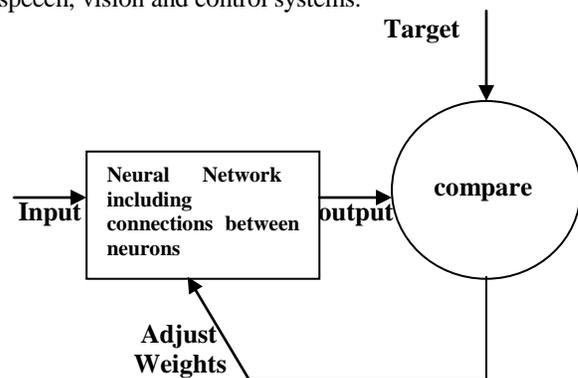
Fig. 1. : Neural Networks block diagram
