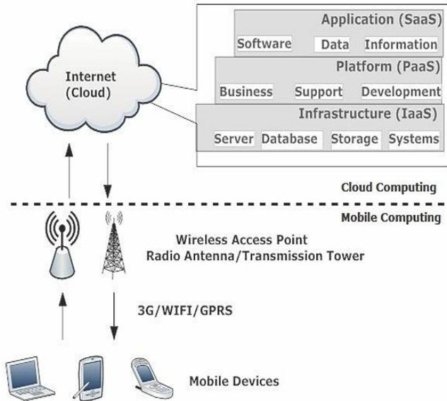
Fig. 3: Architecture of Mobile Cloud Computing
