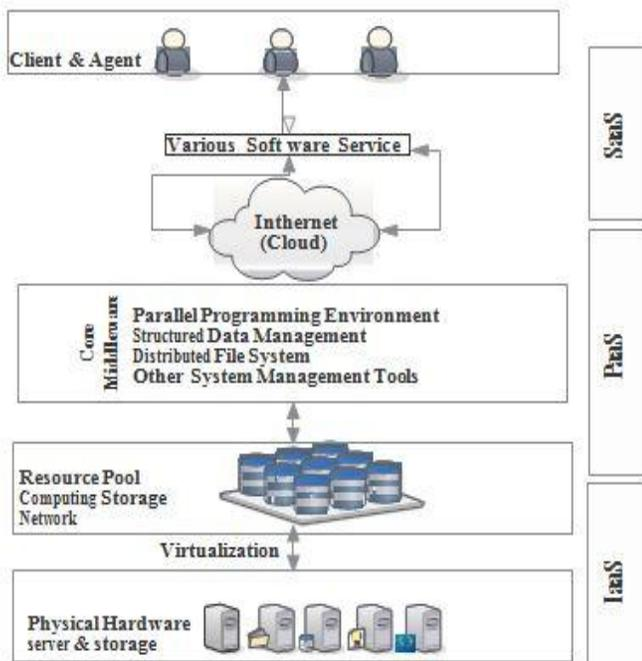
Fig. 2: The Framework of Cloud Computing
